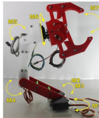
Figure 6. Servo motor movement on the robotic arm
